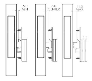
6mm horizontal adjustment can be adjusted after installation 2 x 5mm packers provided (Installation Optional)
